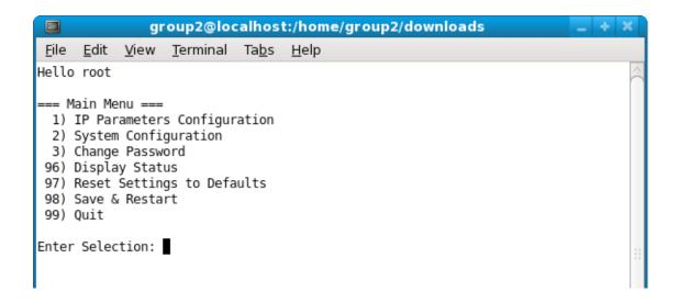
5. When all settings are completed, save the changes using "98( Save and Restart)" - "1(Save & Restart device & Configuration printing)", or "2 (Save & Restart device)". The settings of the printer will be saved. Reset the printer.
