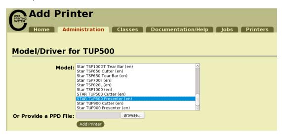
**Caution**: In some versions of CUPS, Star model name is not displayed in the model/driver pull-down menu. In such cases, after performing the following, return to the previous page and reregister the printer.
